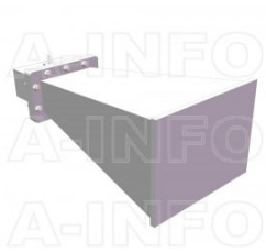
LB-510-10-C-SFSPO Standard Gain Horn Antenna 1.45-2.2GHz 10dB Gain SMA Female
